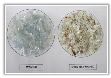
Oven test low level of multilayer
