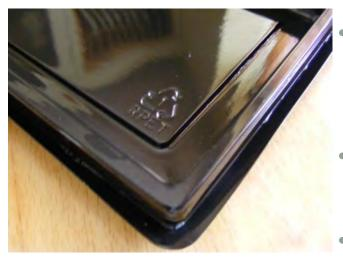
Commercial carbon black trays from UK retailers were tested using NIR, MIR and Laser based Spectroscopy
