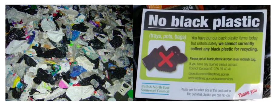
Black pots, tubs and trays are typically colored with carbon black masterbatch based pigments. Carbon black readily absorbs visible and infra-red light.
