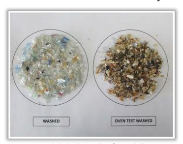
Oven test high level of multilayer
